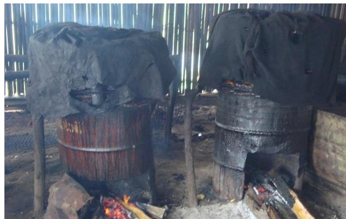
**Plate8.** Traditional Cut-Drum Fish Smoking Oven
